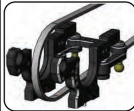
Note : Before assembly please put Midship Belt 354 between Bulkhead A & B to facilitate later drivetrain installation.
