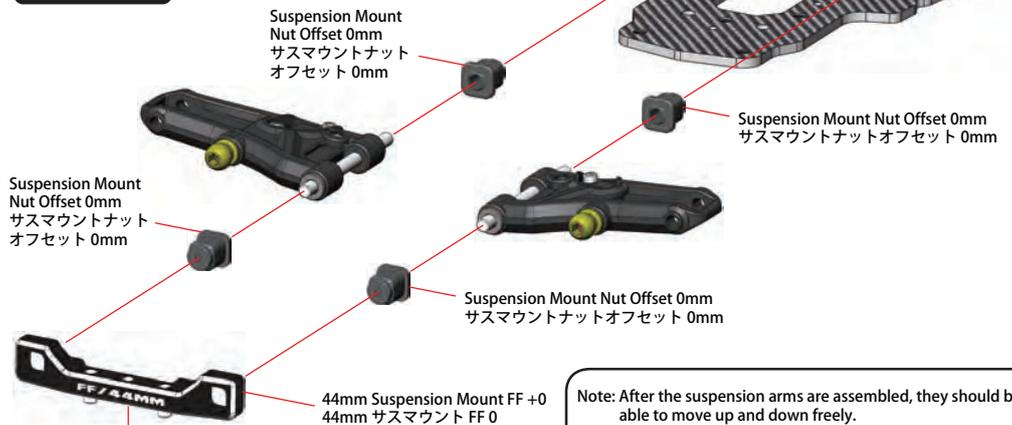
Note: After the suspension arms are assembled, they should be able to move up and down freely.
