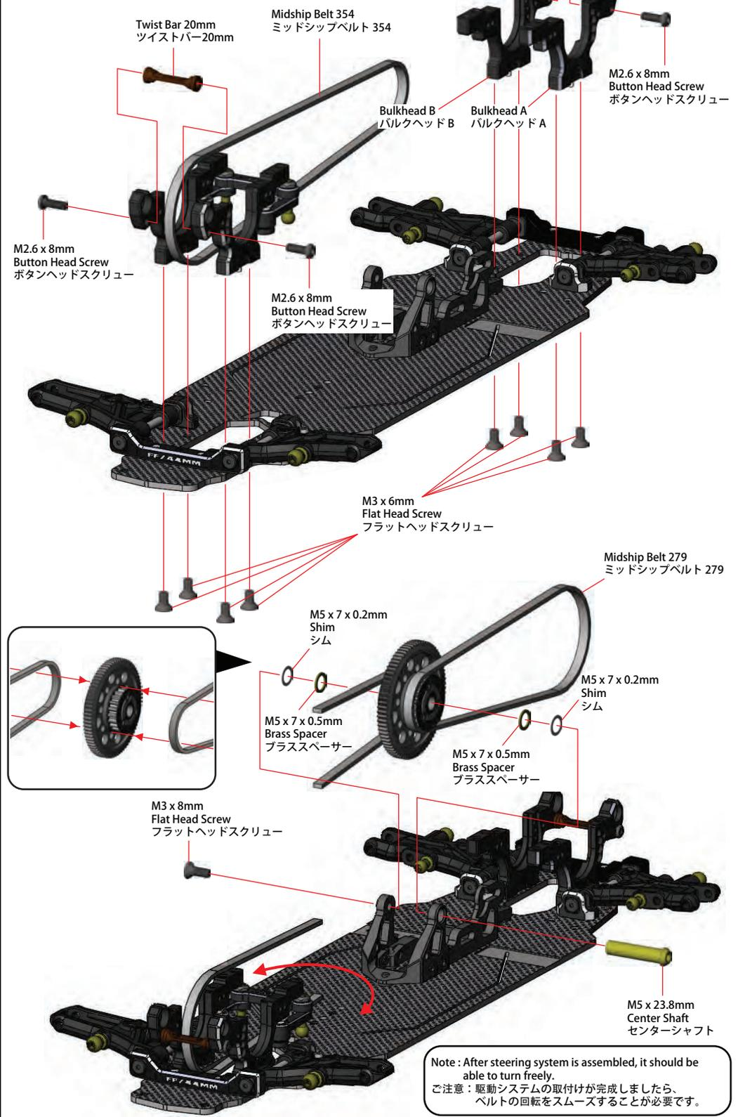
Note : After steering system is assembled, it should be able to turn freely.
