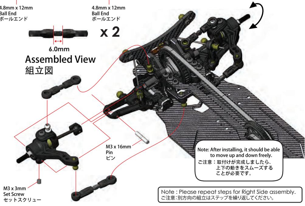
Note: After installing, it should be able to move up and down freely.
